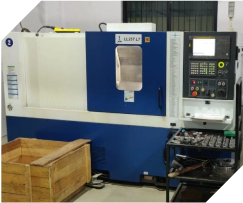
LMW MAKE – LL25T L7 (CNC TURNING) 12" Chuck Size
