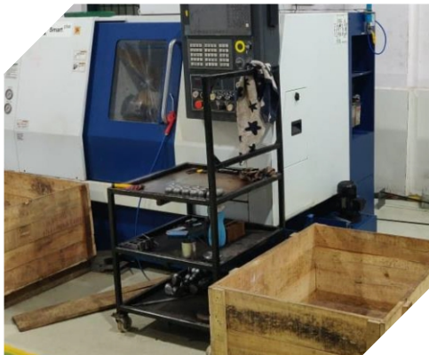
LMW MAKE - SMART TURN PLUS (CNC TURNING) 8" Chuck Size
