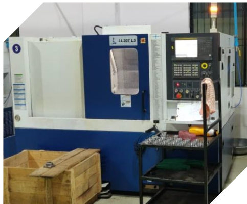
LMW MAKE - LL20T L5 (CNC TURNING) 10" Chuck Size
