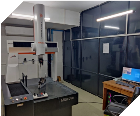
CMM MITUTOYO CMM CRYSTA-APEX V WITH UNIVERSAL RENISHAW PROBE. Size : X-700mm x Y-1000mm x Z-600mm
